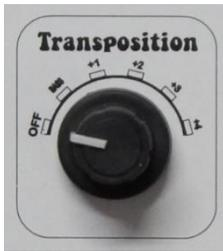
The term transposition is a musical term and refers to the equal raising of a note or sequence of notes. The transposition switch of the Thor theremin model has 5 possible settings (plus ON/OFF). The leftmost setting, "Bass", is the lowest possible range of the theremin. In relation to this setting, the pitch is raised by approx. 1 octave at "+ 1". Correspondingly, the other 4 possible settings raise the pitch by 2, 3, 4 or 5 octaves.
