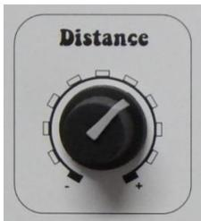
The theremin has a Distance control on the top of the unit and a distance adjustment control on the bottom of the unit. Both distance controls have the same function, but the control on the top of the unit allows fine adjustment.
