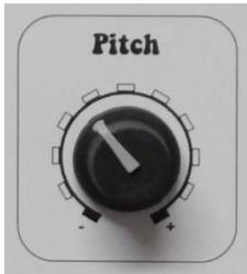
The theremin has a pitch control on the top of the unit and a pitch adjustment control on the bottom of the unit. Both pitch controls have the same function, with the control on the front of the unit providing fine adjustment.
