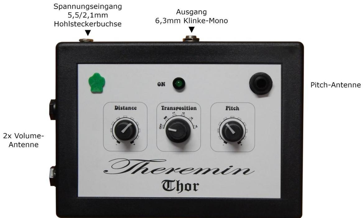
The theremin is played by the approach and distance of the player's hand. The following applies: The further the hand is removed from the antenna, the deeper the sound.
